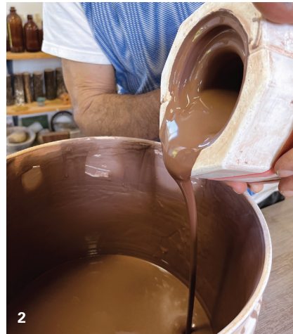
2 After about 20 minutes, drain the mold and leave it upside down for approximately 10–15 minutes.
