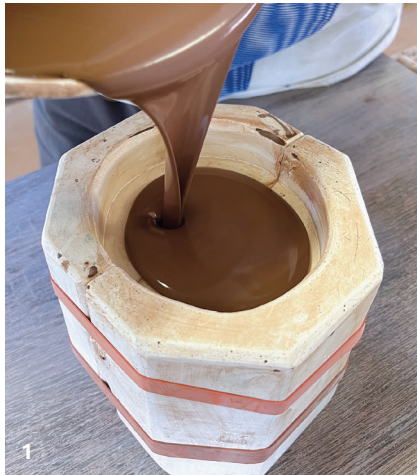
1 Pour a red-earthenware casting slip into a dry plaster mold to create a small oval-shaped cup.
