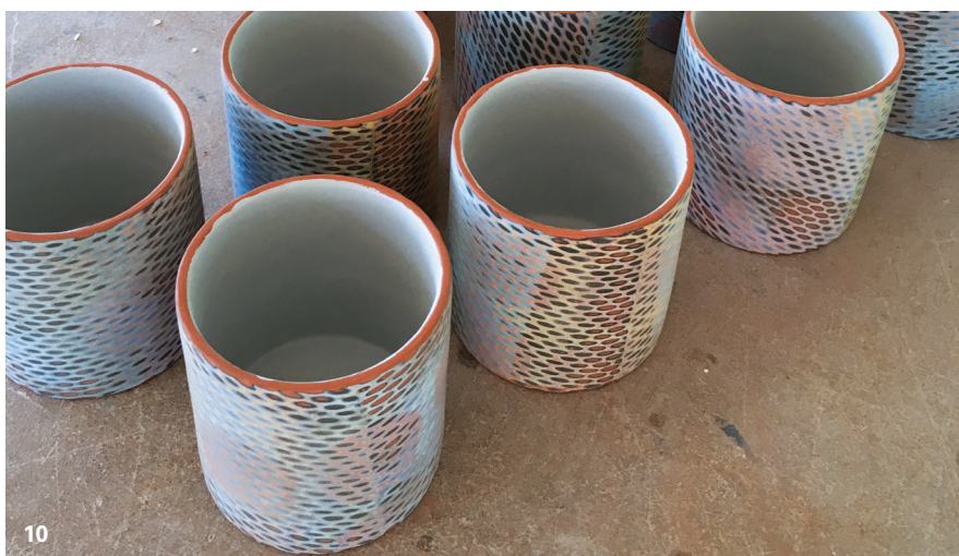
10 Bisque-fired mugs with liner glaze. Note the orientation of the plastic mesh can be rotated to create a variation of the etched pattern.
