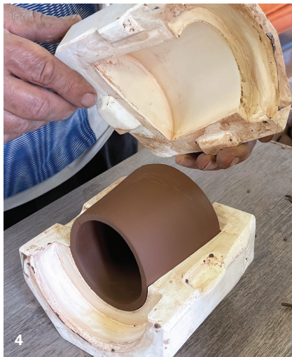
4 Remove the piece from the mold, leave it to dry, then clean up the seams.
