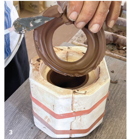
3 Trim the reservoir away, then allow the piece to firm up until it pulls away from the mold.
